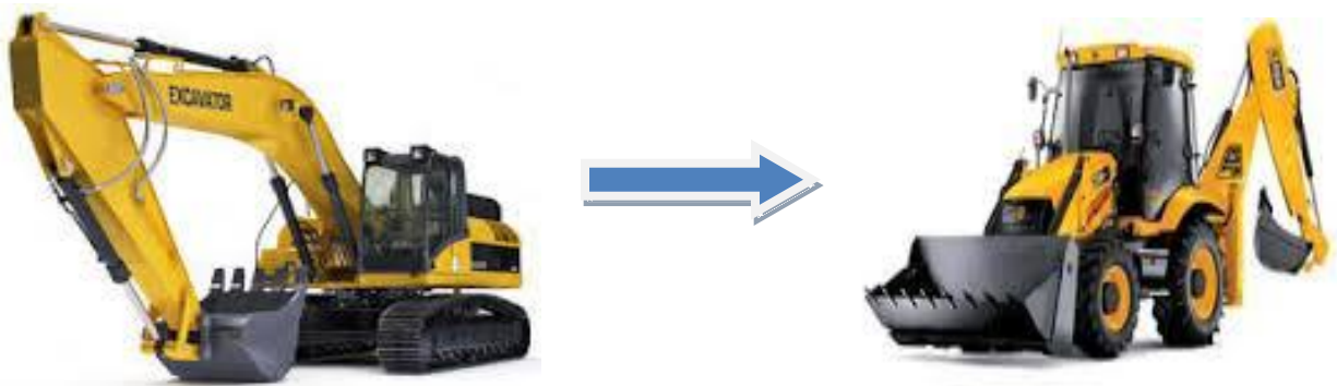
Fig 5.5 Excavator 0.5cum capacity upgraded to 1 cum capacity
