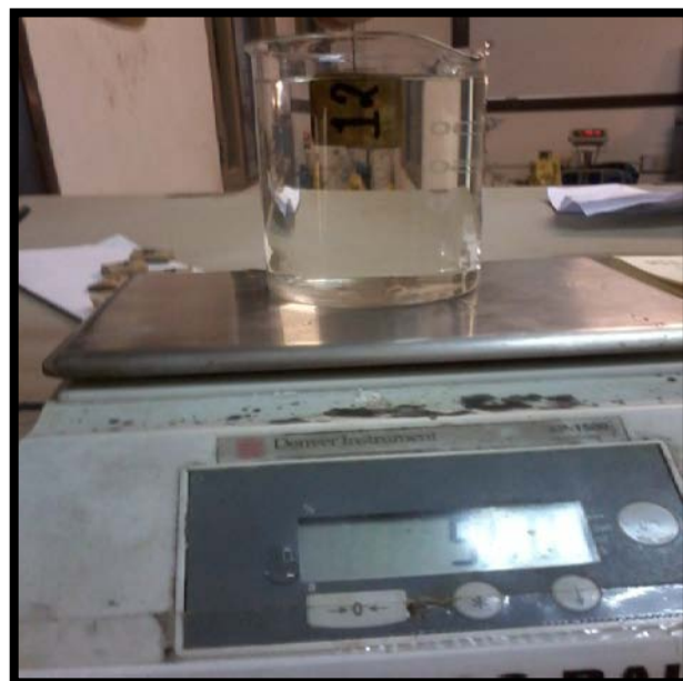
Figure 2: Water displacement method for determining the green volume
