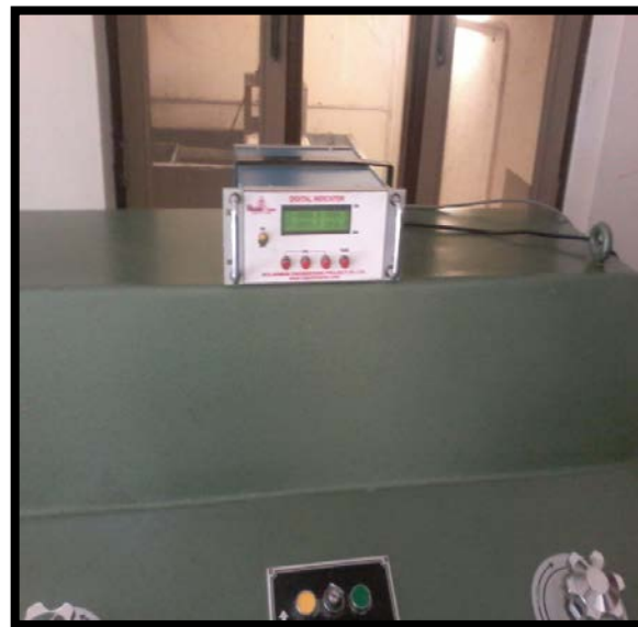
Figure 12: Digital indicator of UTM, displaying the load and displacement readings.
