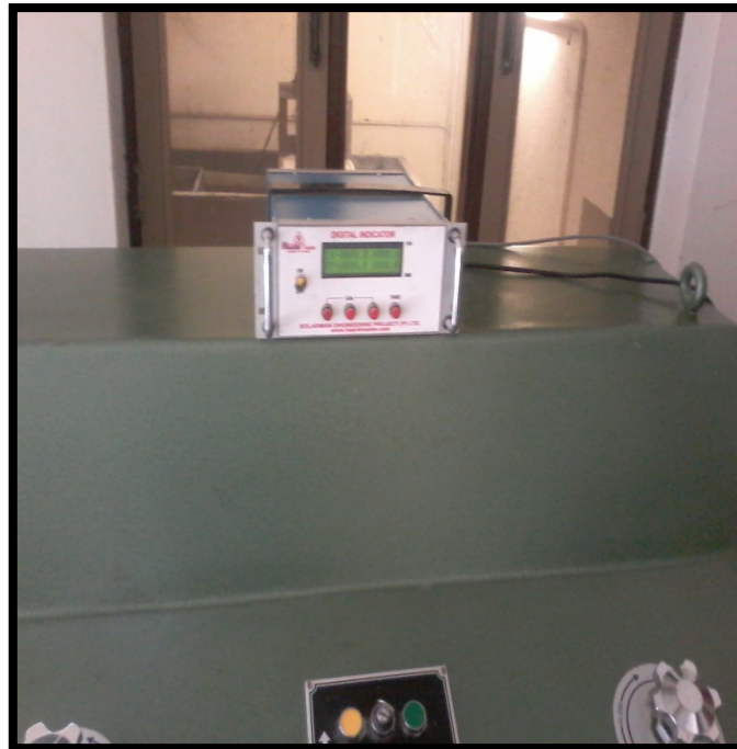
Figure 15: Digital indicator of UTM, displaying the load and displacement readings.
