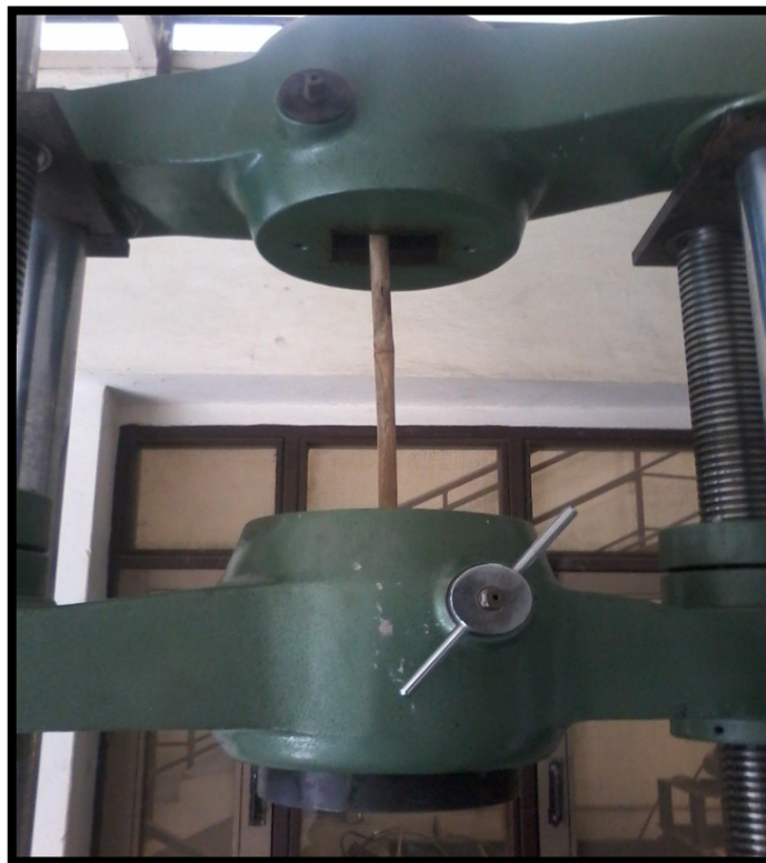
Figure 14: Application of tensile load on samples, on a UTM
