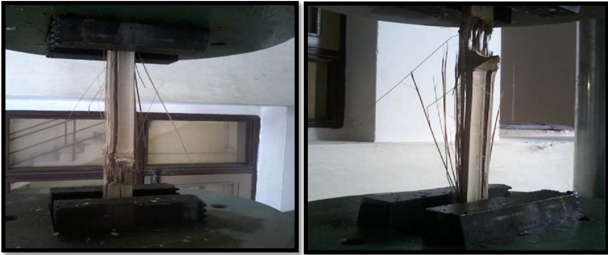
Figure 25: Brittle Failure of bamboo splint at node under tensile load.
