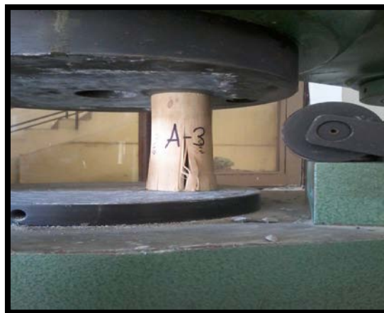
Figure 22: Cracking as well as crushing of fibers
