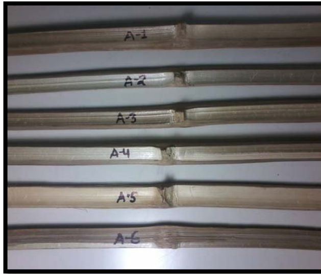
Figure 13: Samples for Tension test
