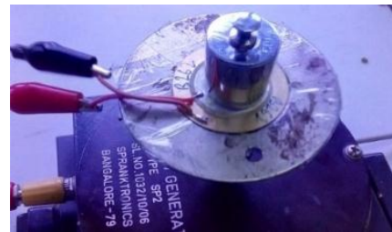
Fig. 1. The fixture with the piezo buzzer and mechanical load attached
