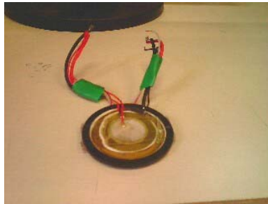
Figure 9 A stack of four piezo discs connected in parallel (see online version for colours)
