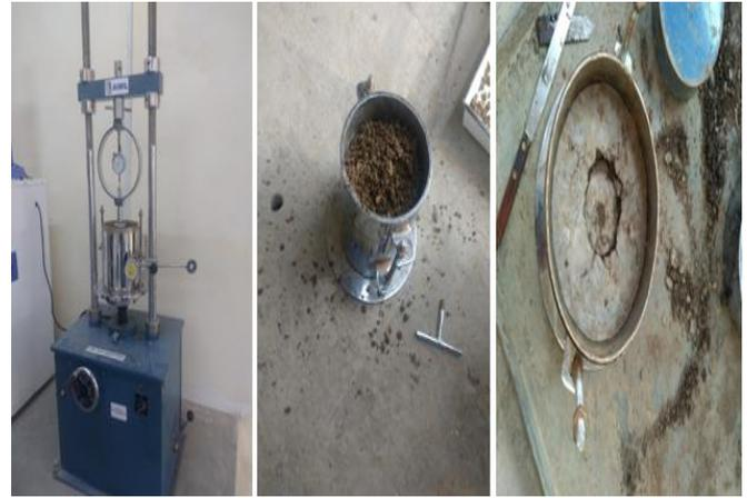
Fig. 5. California Bearing Ratio Test in Laboratory
