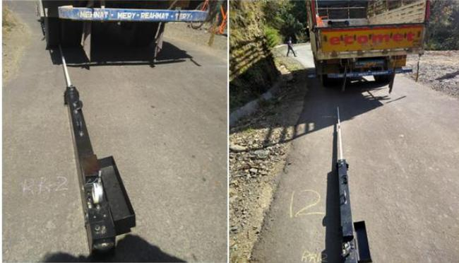
Fig. 3. Benkelman Beam Deflection study on selected stretches
