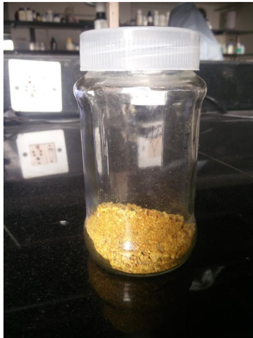
Figure 3.1. Orange pomace dried to utilize it as a solid substrate in SSF
