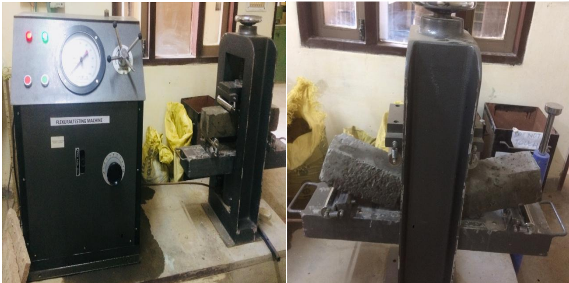
FIGURE 4.15 TESTING OF BEAM IN FTM
