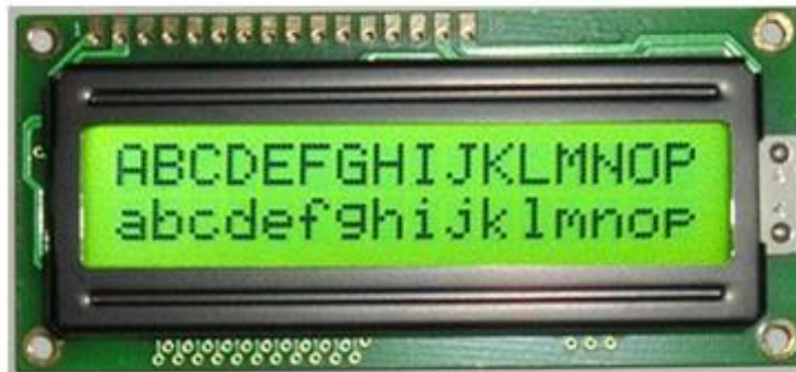
Figure 3.6 Dot Matrix LCD [10]
