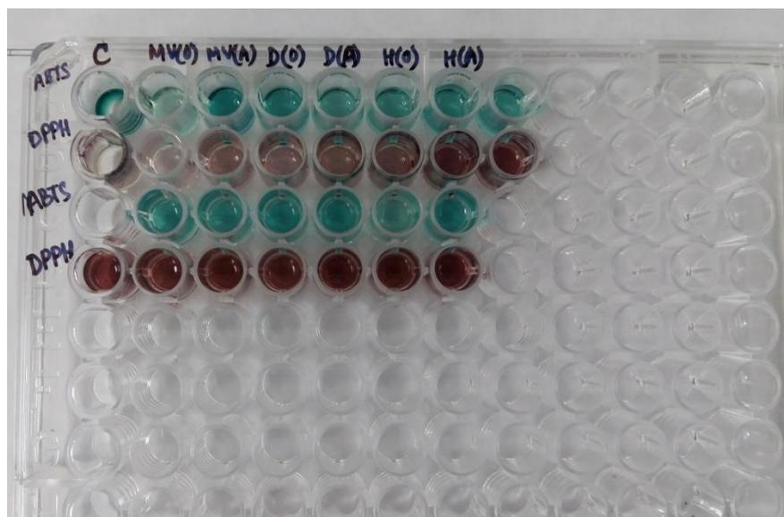
Figure 5.1: The changing color of samples containing ABTS and DPPH in different concentrations
