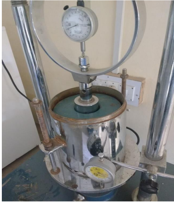
Figure 2.6: Testing on CBR sample
