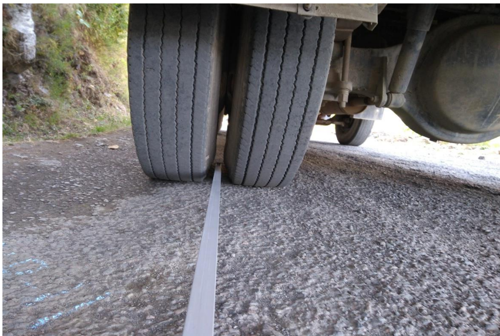
Figure 3.5: Placing of probe of the benkelman beam
