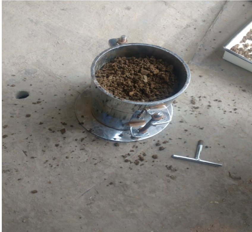
Figure 2.5: Mould filled with CBR sample
