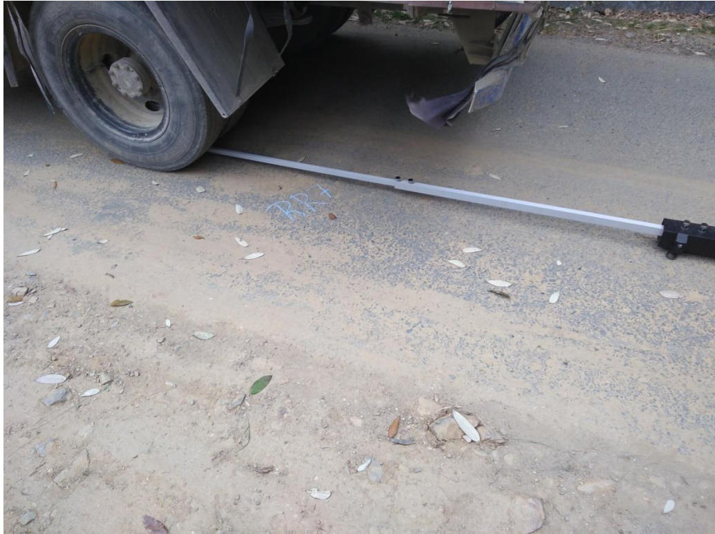
Figure 3.2: Placing of benkelman beam between the tyres at RR 7
