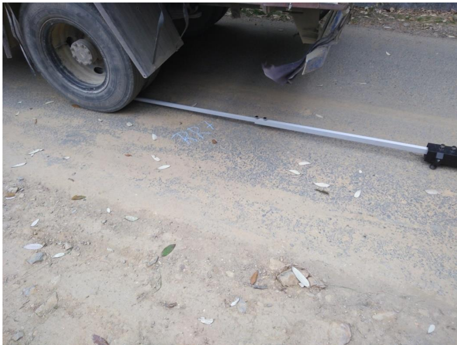
Figure 1.3: Placing of the benkelman beam
