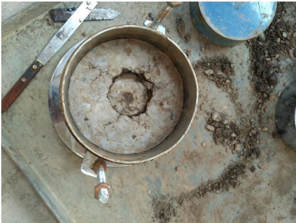
Figure 2.7: Soil sample failure after CBR test
