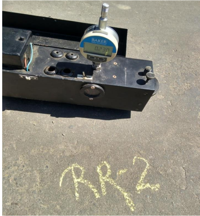
Figure3.6: Benkelman beam reading at RR 2
