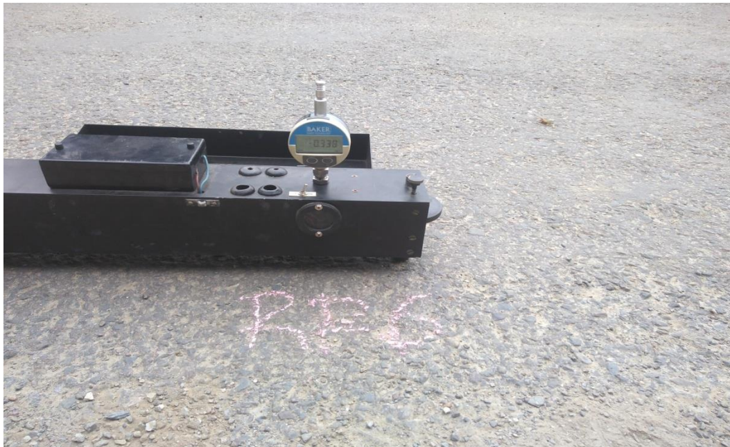
Figure 3.3: Deflection reading when truck moves 2.7 metres from initial position
