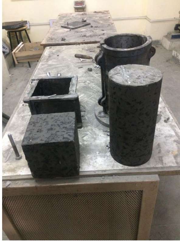
Figure 3. 1 concrete cube and cylinder with 10% replacement of WFS & WCT
