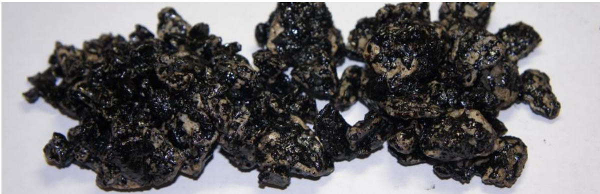
Fig. 23- Aggregates coated with bitumen after the test
