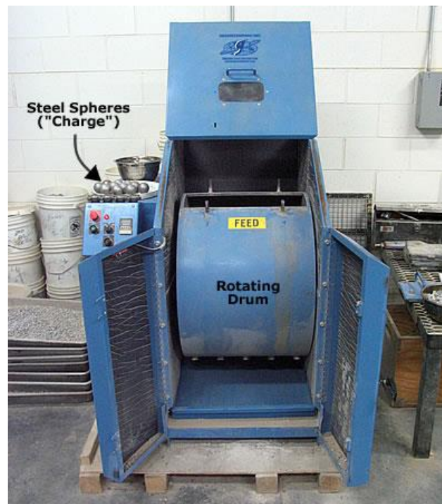
Fig. 10-Los Angeles Abrasion Value Test Apparatus
