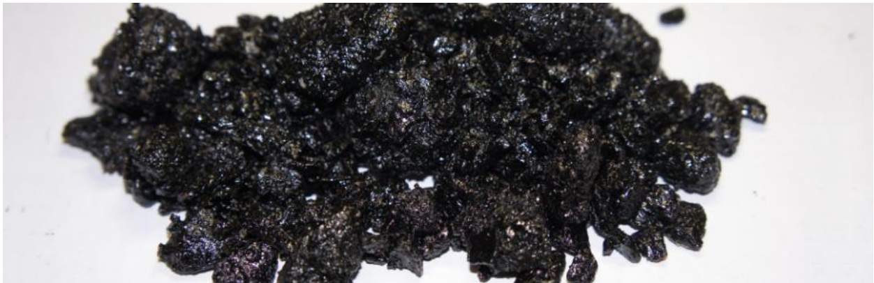
Fig. 36- Aggregates coated with bitumen modified with Zycotherm after test
