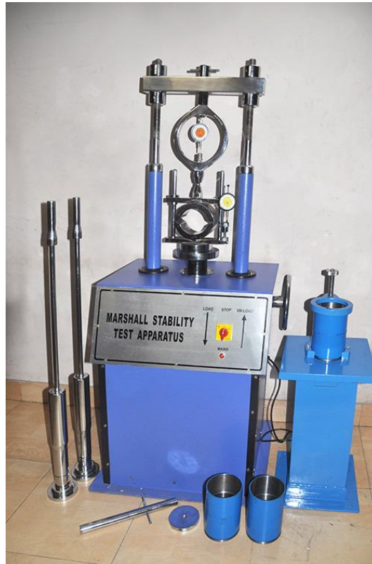
Fig. 21-Marshall Stability Test Apparatus
