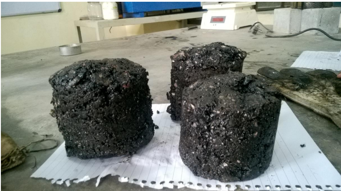
Fig. 35- Sample after Testing (Bulging Failure)
