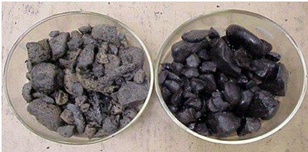
Fig. 22-Image Showing Stripping of Bitumen from Aggregates
