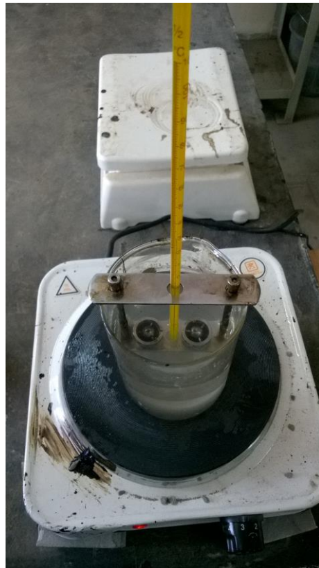
Fig. 18-Ring and Ball Apparatus
