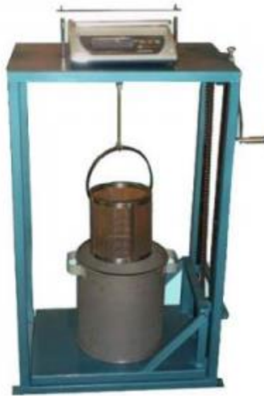
Fig. 11-Specific Gravity Frame and Basket
