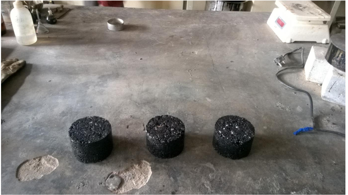
Fig. 31- Bituminous concrete mix samples
