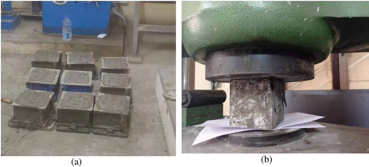
Fig 3.13 (a) Compressive Strength Casting (Cube-15cm*15cm*15cm) (b) Compressive testing using UTM
