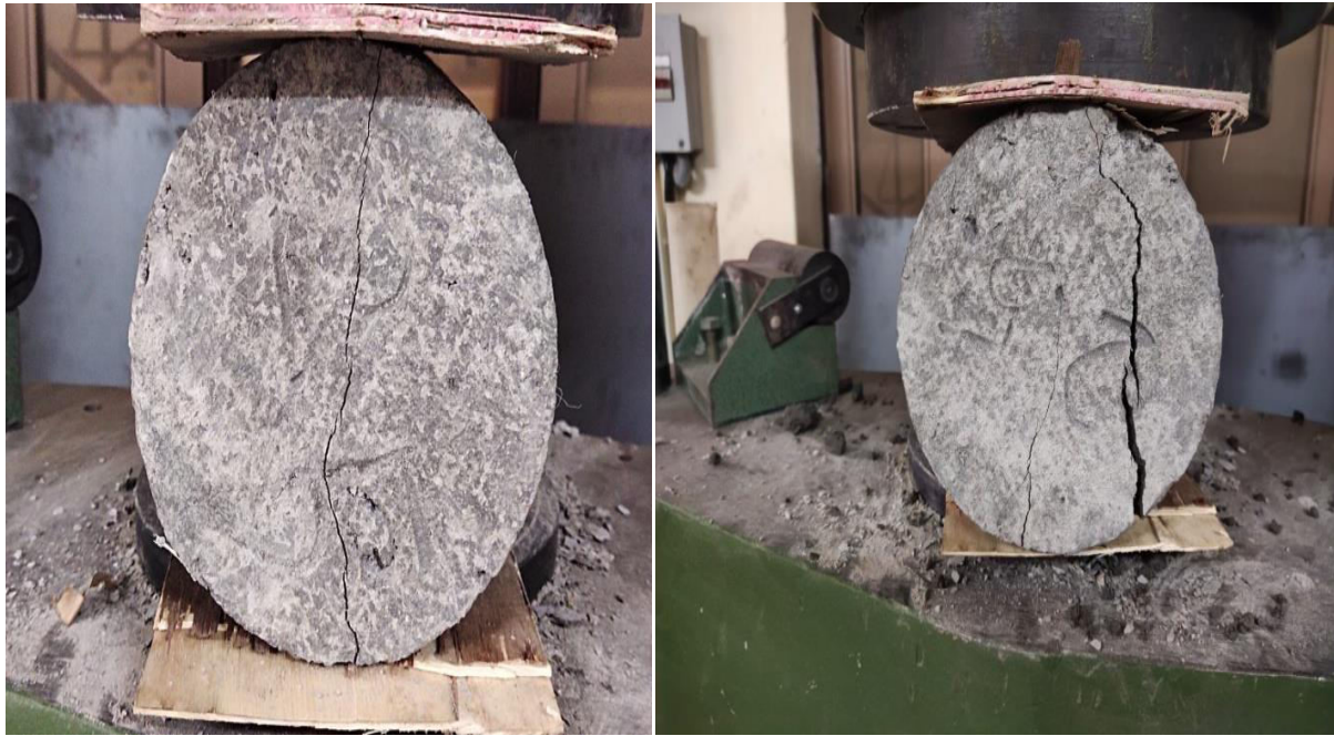
Fig 3.15 Split Tensile Strength Testing using UTM (Cylinder, h=30cm, d=15cm)
