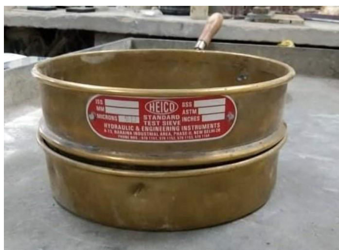
Fig 3.4 Sieve Analysis (90 \mu ).
