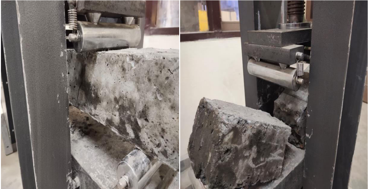
Fig 3.14 Flexural Strength Testing using third point loading
