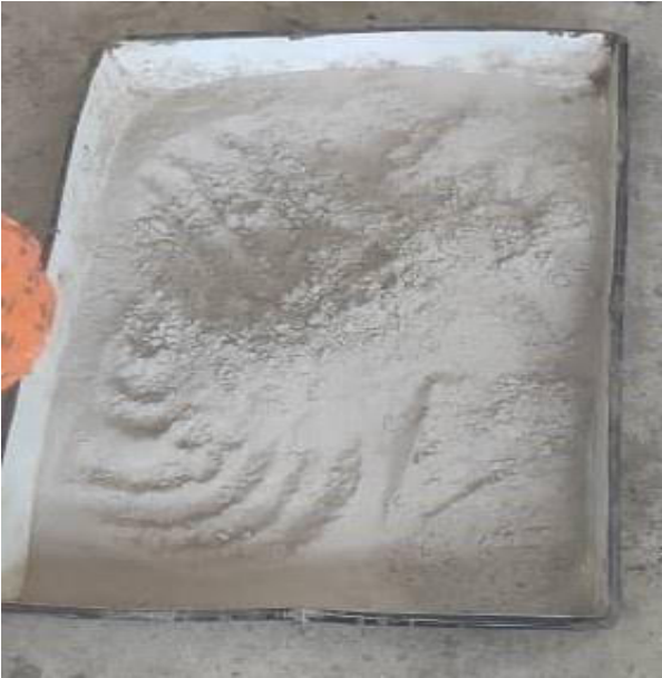
Fig 1.1 EAFS Passing 90 \mu Sieve.
