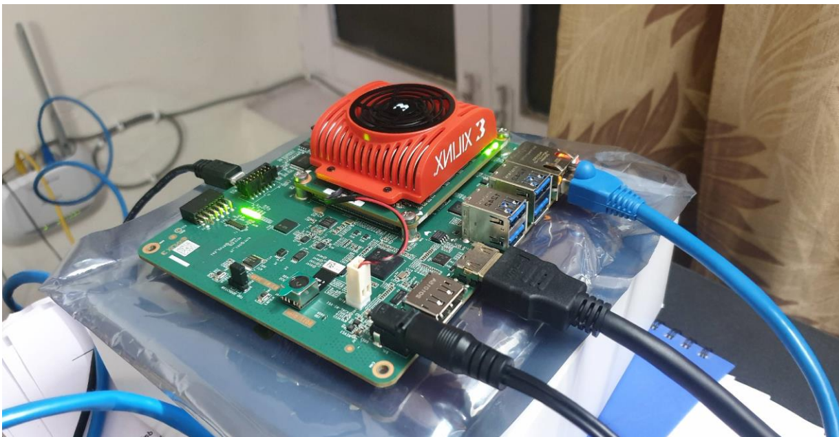
Fig 3.2.1b: Actual Kria KV260 board Connected to PC
