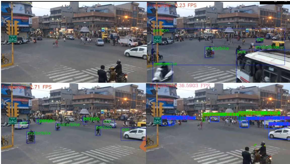
Fig 4.7.1b : 4 screen Grid of output of different hardware inference of sample 2. Top left screen is the original video. Top right screen is output of CPU inference. Bottom left is output of GPU inference. Bottom right is the output of FPGA inference.
