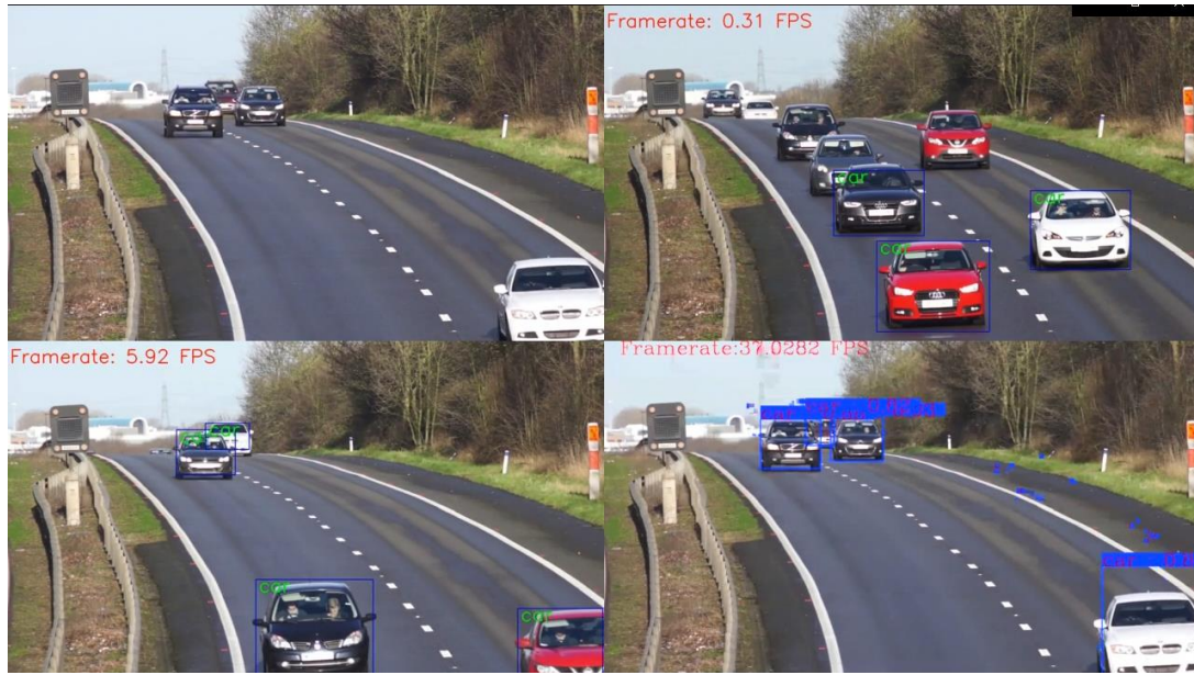
Fig 4.7.2a : 4 screen Grid of output of different hardware inference of sample 5. Top left screen is the original video. Top right screen is output of CPU inference. Bottom left is output of GPU inference. Bottom right is the output of FPGA inference.
