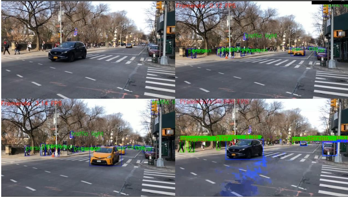
Fig 4.7.1a : 4 screen Grid of output of different hardware inference of sample 1. Top left screen is the original video. Top right screen is output of CPU inference. Bottom left is output of GPU inference. Bottom right is the output of FPGA inference.
