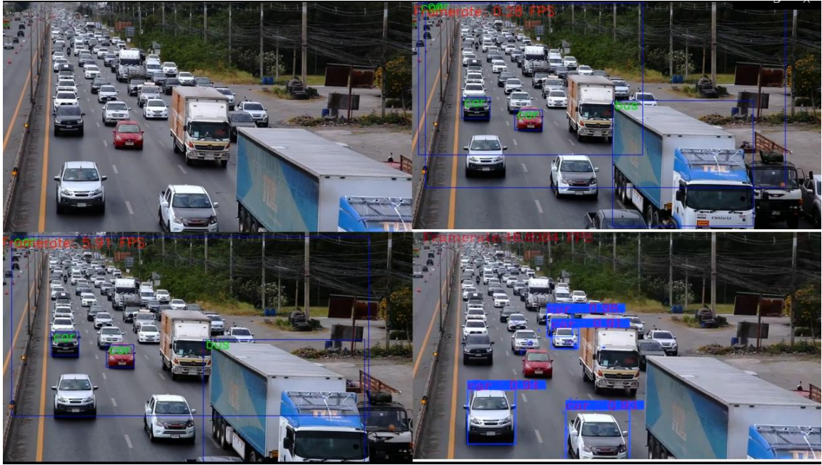
Fig 4.7.1c : 4 screen Grid of output of different hardware inference of sample 3. Top left screen is the original video. Top right screen is output of CPU inference. Bottom left is output of GPU inference. Bottom right is the output of FPGA inference.
