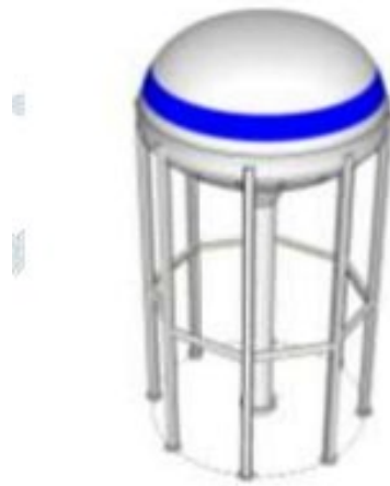
Figure (7): Spherical type water tank
