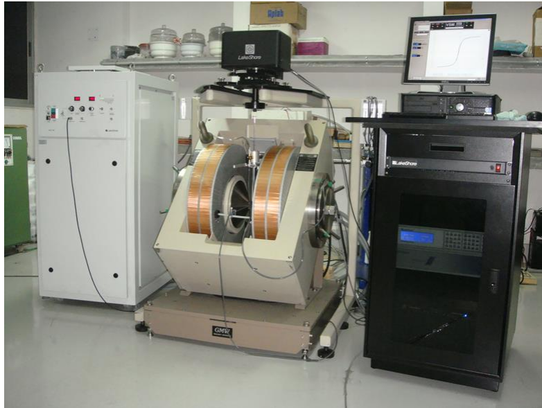
Figure 2.17: Picture of “Vibrating sample magnetometer model PAR-155”
