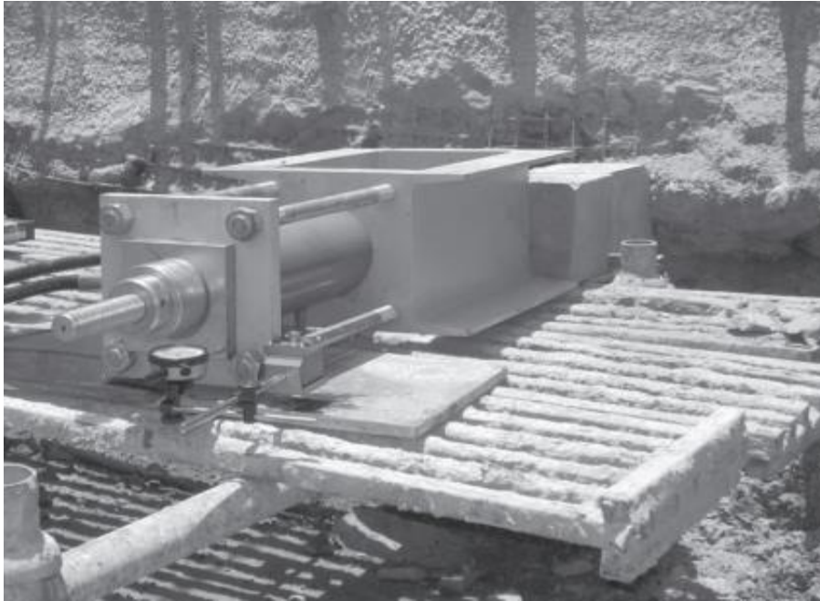
Fig.2. 34 Field pullout test [63]
