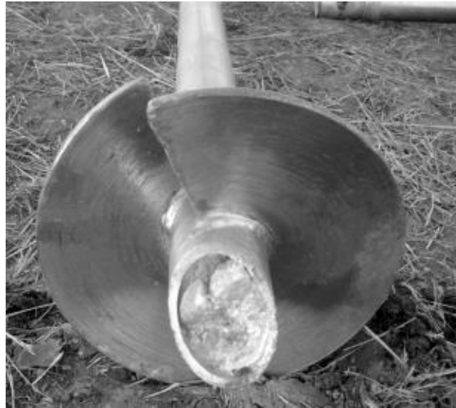
Fig.2. 45 Plugged end of a typical helical pile (Perko, [9])
