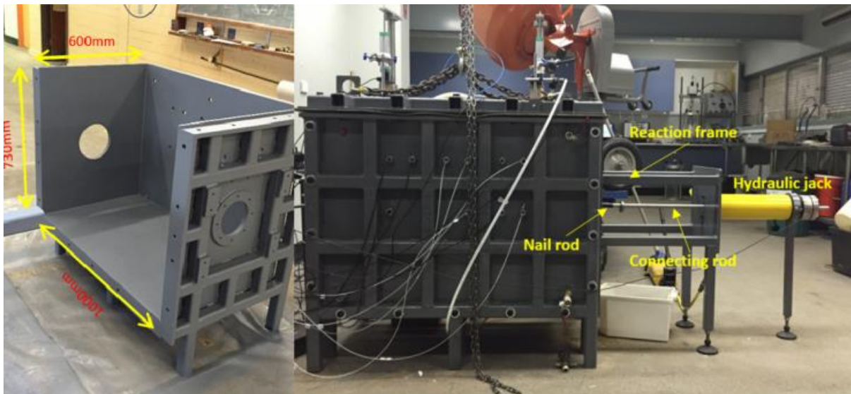
Fig.2. 29 The laboratory pull-out system (Ye et al. [59])
