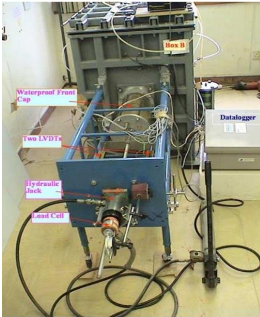
Fig.2. 22 laboratory pullout setup of Yin and Su [55]
