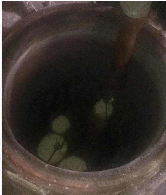
Figure 3.14 CFST specimens in heating furnace for annealing
