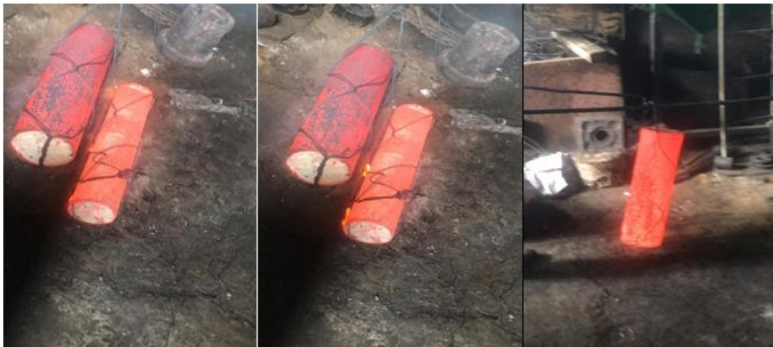
Figure 3.17 CFST columns after heated at elevated temperature of 600 °C & 800 °C
