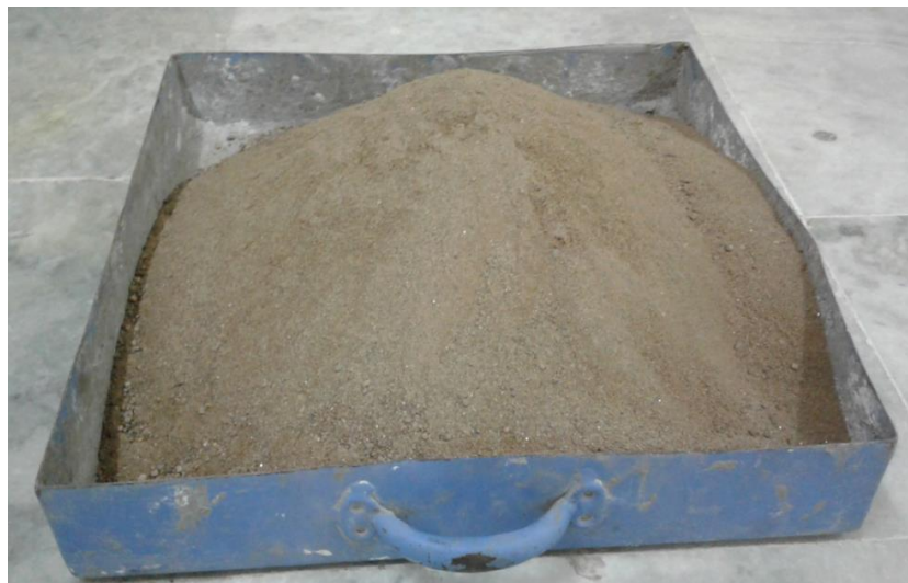
Figure 3.3 Sample of Fine aggregate passed through 4.75mm sieve
