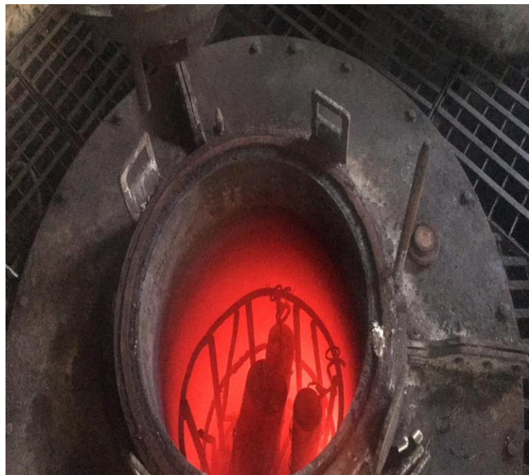
Figure 3.10 CFST specimens placed in heating furnace
