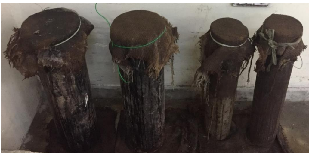
Figure 3.8 CFST specimens closed with wet burlap
