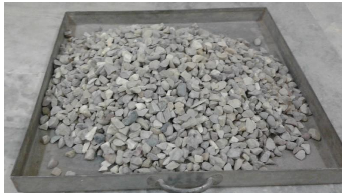
Figure 3.2 Sample of coarse aggregate pass from 20mm sieve
