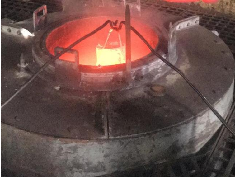
Figure 3.13 CFST specimens pulled outside after reached target temperature
