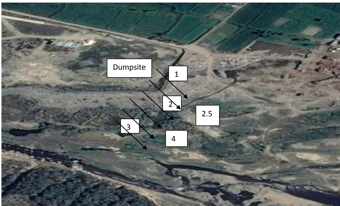
Figure 8.1(d): Location of Baddi dumpsite and groundwater sampling points
