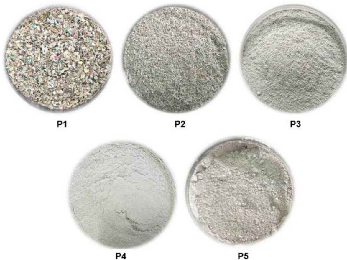
Figure 3.2: Pulverized CPCBs of different particle sizes: P1) \geq 0.71 mm; P2) 0.35 to 0.71 mm; P3) 0.15 to 0.35 mm; P4) \leq 0.15 mm and P5) \leq 0.15 mm
