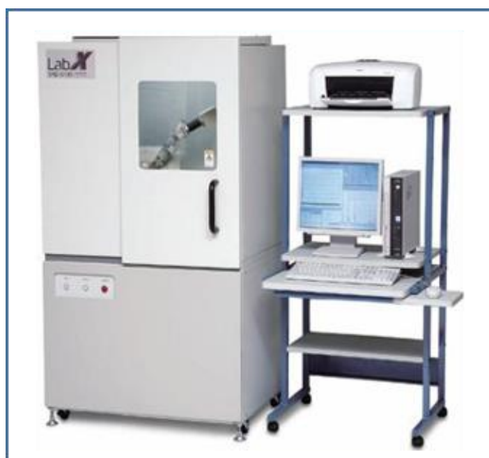
Figure 2.6: Photograph of X-ray diffractometer Shimadzu-6000 model.
