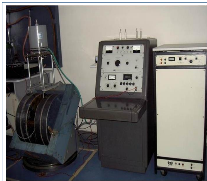
Figure 2.13: Photograph of vibrating sample magnetometer model PAR-155.
