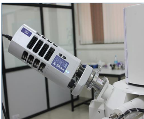
Figure 2.10: Photograph of oxford instruments EDX.
