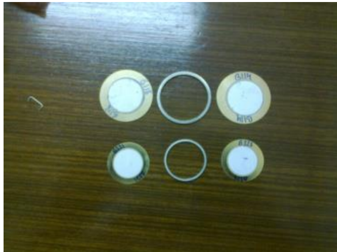
Figure 3.12 The piezoelectric buzzer elements with steel rings
