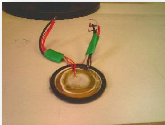
Figure 2.9 Stack of four Piezo Discs connected in parallel
