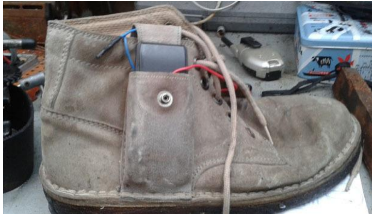
Figure 2.5 Quartz crystal powered shoe generator designed by Trevor Baylis
