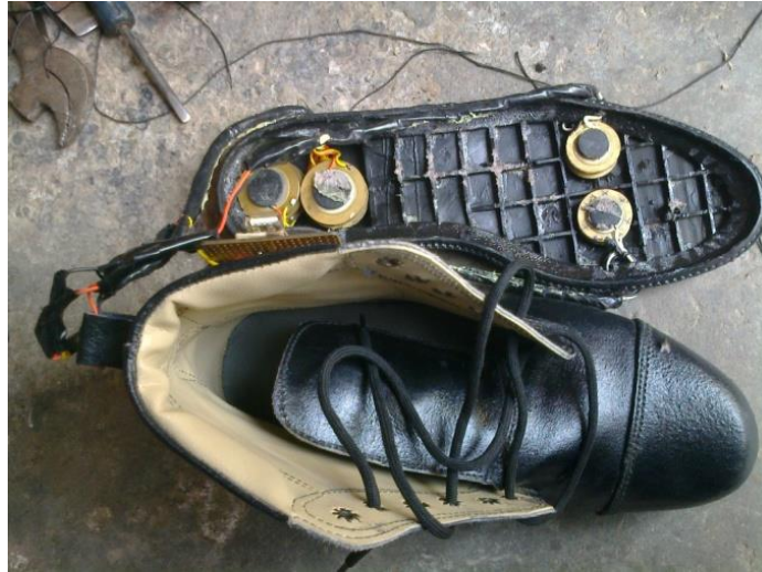
Figure 3.26 DMS shoes with energy harvesting stacks embedded in the heel and forefoot sections (M1).
