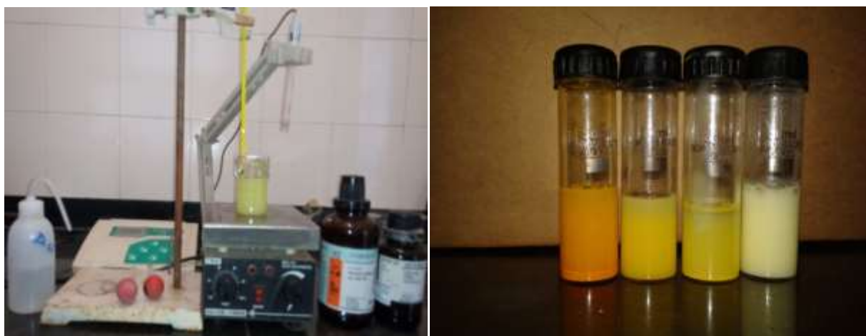
Figure 2.2: Experimental arrangements employed for wet chemical synthesis of CdS QDs, right side picture shows different size QDs.
