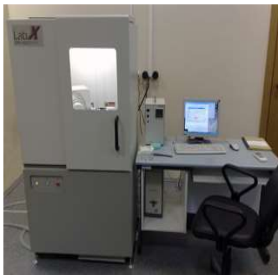
Figure 2.5: Shimadzu (XRD 6000) X-Ray diffractometer employed for XRD experiments.
