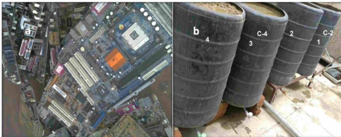
Figure 3.5: (a) E-waste used in column leaching, (b) Column leaching procedure adaptation to determine the actual hazardous metal leaching to land system
