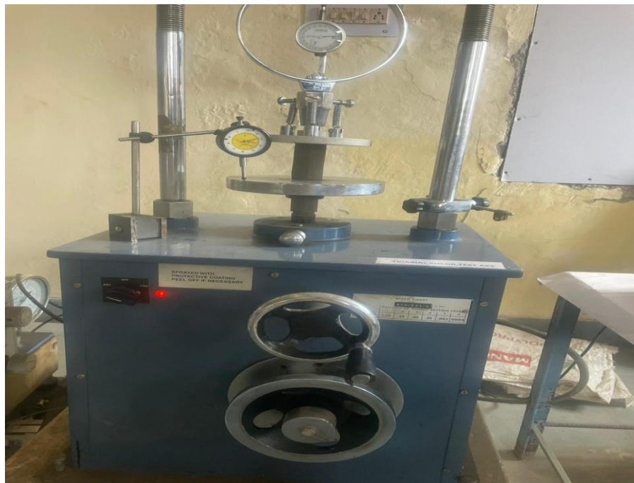
Figure 4.2 : UCS testing of soil sample
