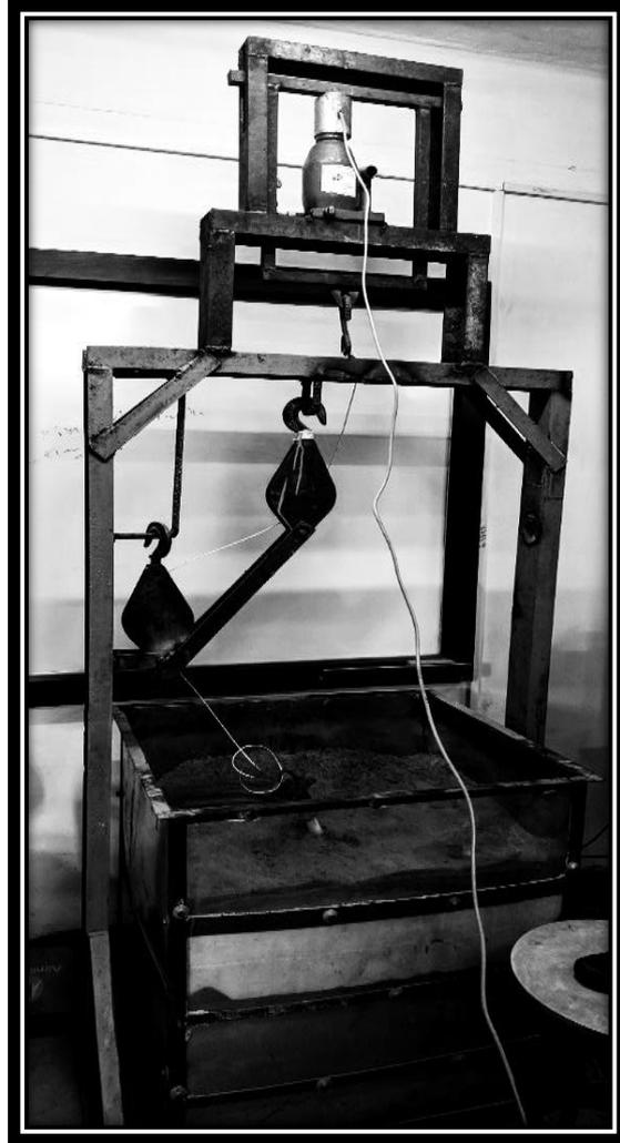
**Figure 3.19** Hydraulic Jack alongwith load cell on test frame
