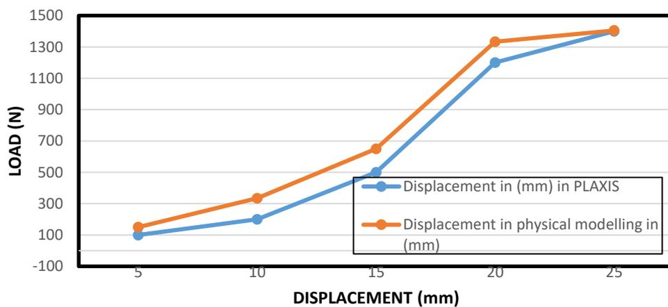
Figure 4.4 L-D curve for three 520 mm Piles
