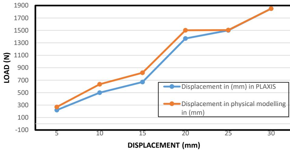
**Figure. 4.5** L-D curve for three 646 mm Piles
