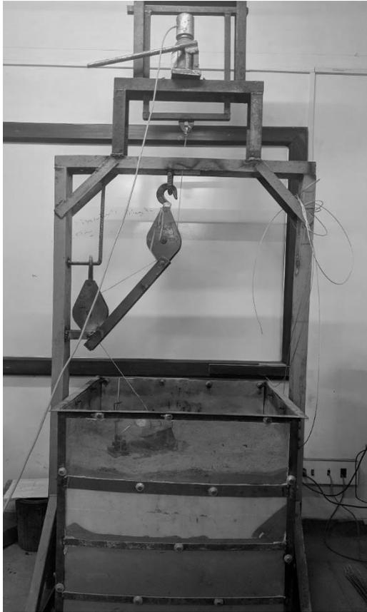
**Figure 4.6** Pull-out test (inclined) performed on 4 PILES
