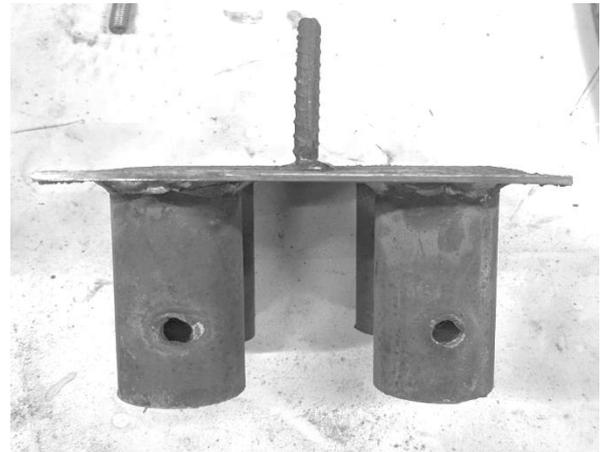
**Figure 3.9 (b)** Pile Cap for four pile arrangement
