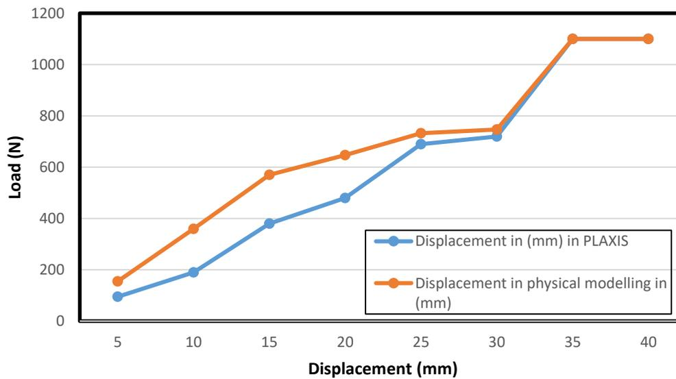
Figure 4.3 L-D curve for 646 mm Pile
