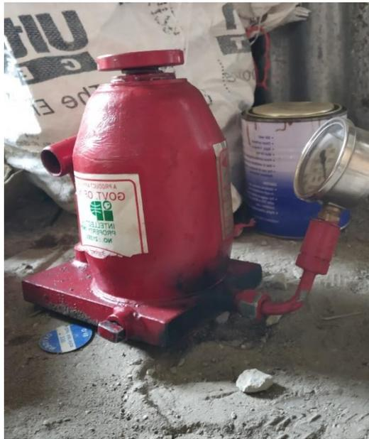
**Figure 3.14** Hydraulic jack used for physical modelling
