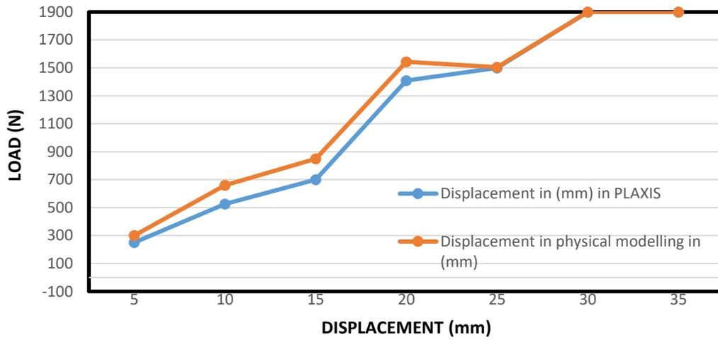
**Figure 4.7** L-D curve for four 646 mm Piles
