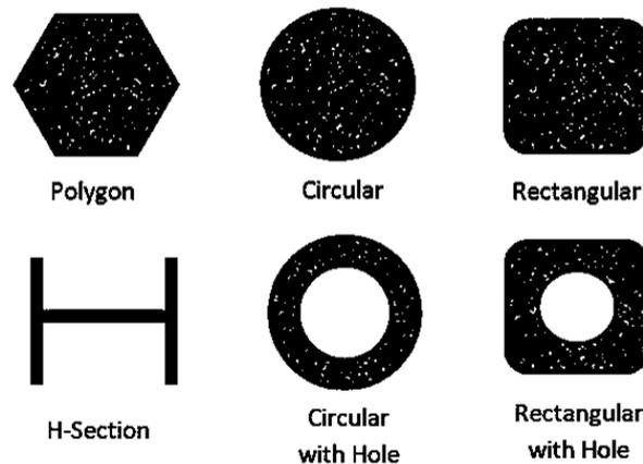
**Figure 1.2** Common shapes of Piles
