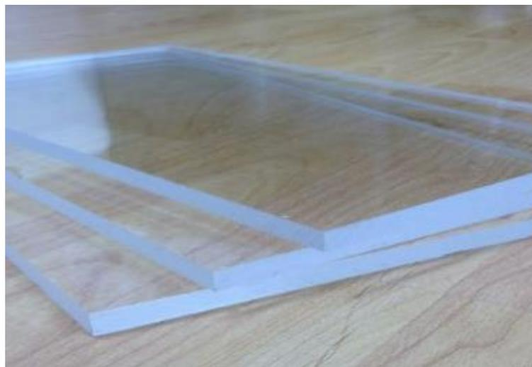
Figure 3.10 Perspex fiber Sheet (0.25 cm)
