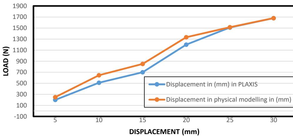
**Figure 4.8** L-D curve for four 520 mm Piles
