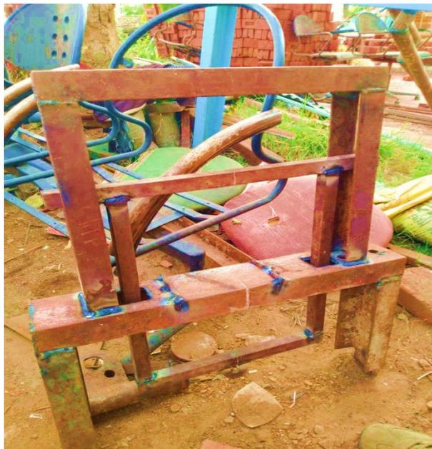
**Figure 3.15** Casing welded for placing the Jack
