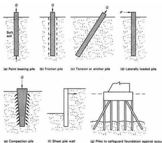
Figure 1.1 Different types of piles
