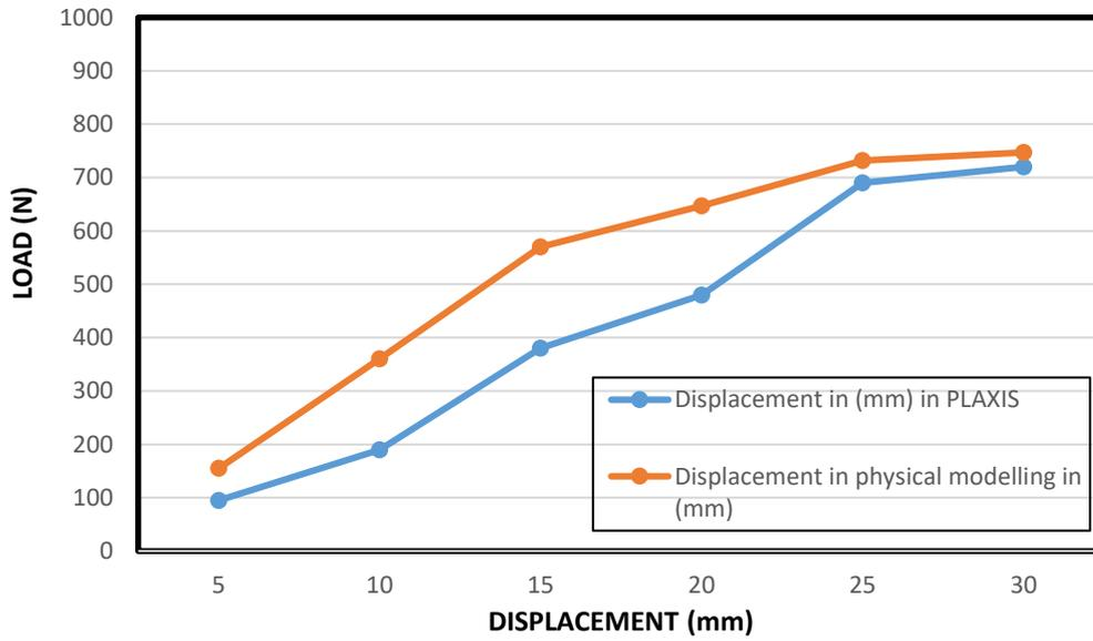
Figure 4.2 L-D curve for 364 mm Pile
