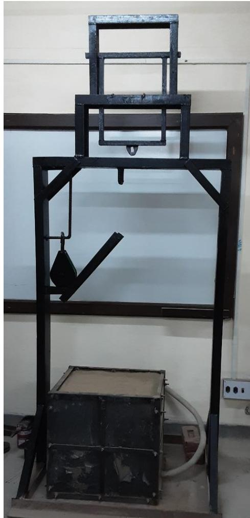
Figure 3.17 Model Tank used for physical modelling
