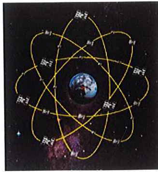
Figure 2.1: Space segment of GPS.
