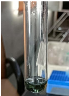
Fig8. Protein concentration using Bradford reagent
