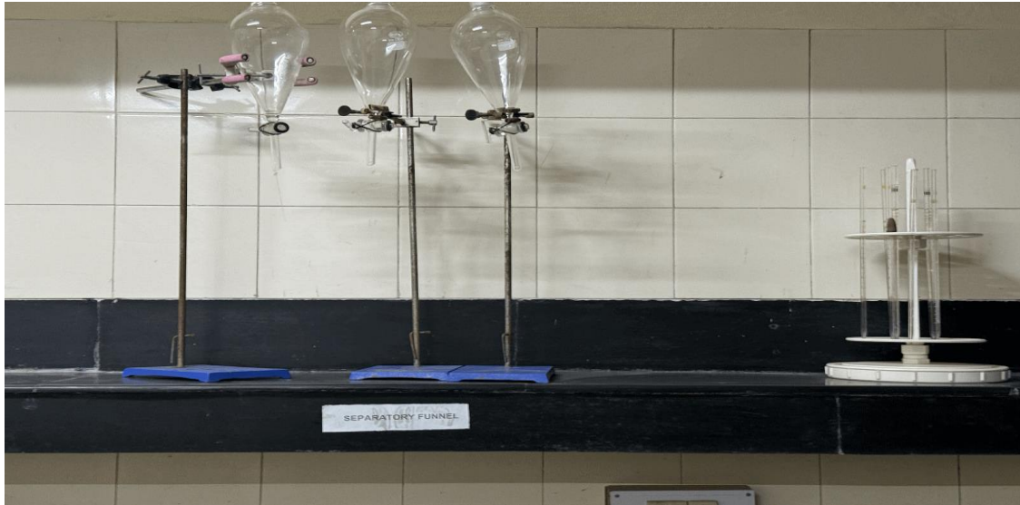
Figure 3.9: Separatory funnel Oil & grease
