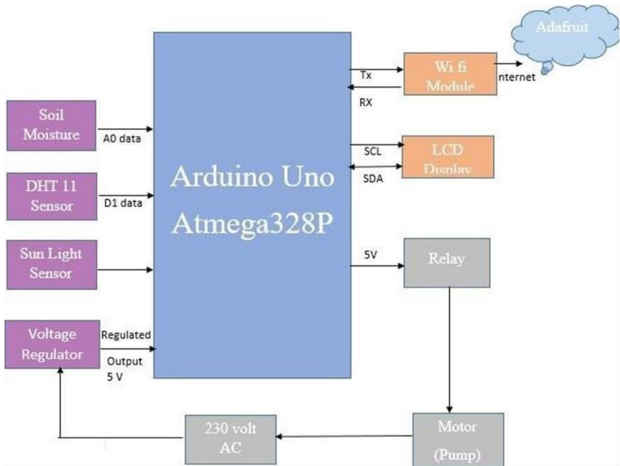
Fig 3: Attached Sensors with Arduino Uno Atmega328P [24]
