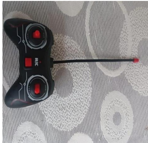
Fig.5&6- R/C car transmitter and receiver of 20 MHz frequency
