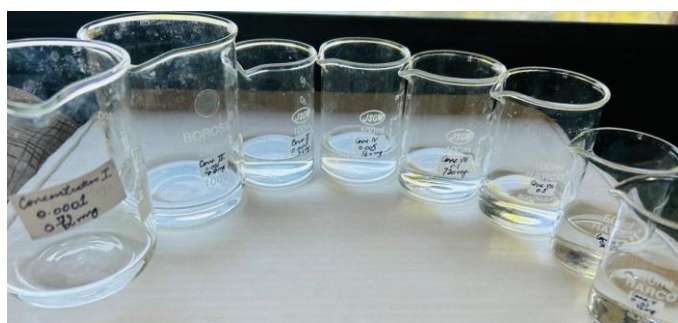
Fig 36. SDS at different concentration for measuring the contact angle
