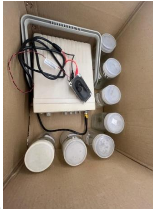
Fig 11. In - vitro plant under acoustic setup of sound waves
