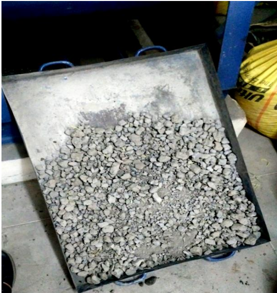
Figure 5: Recycled Aggregates before water-wash and grading
