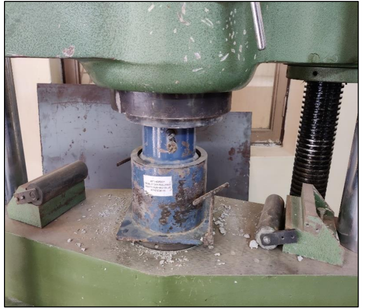
Figure 12: Crushing Strength test
