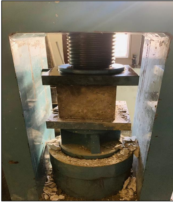
Figure 15: NA testing at 7 days
