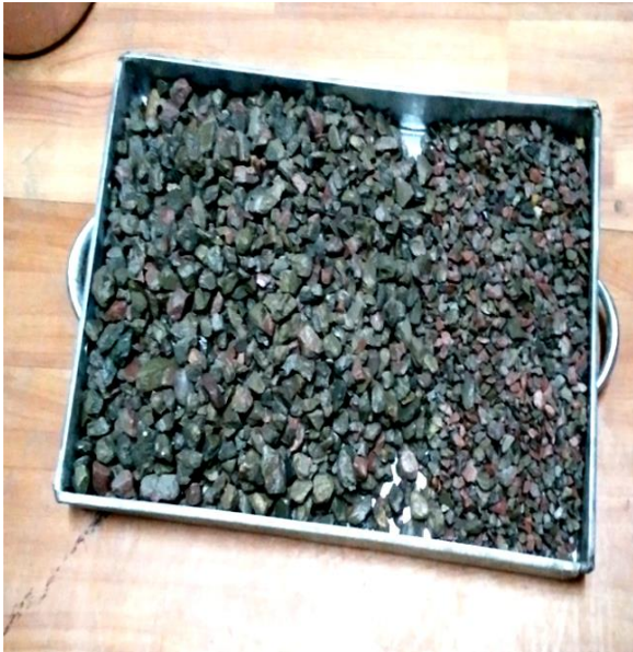
Figure 6: Processed Recycled Aggregates after water wash
