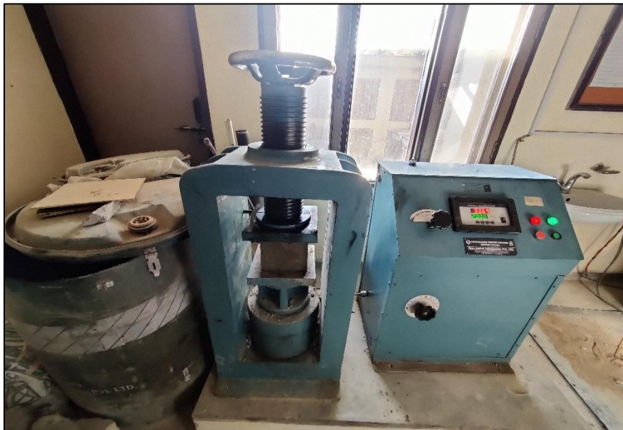
Figure 17: Compressive Strength test on Samples
