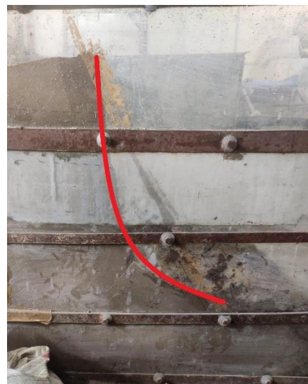
Figure 4.5 (b) Side view of model after failure
