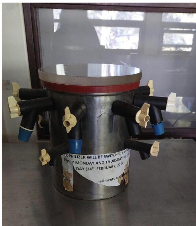
Fig 4.7 - Lyophilizer used for the drying of the extracts
