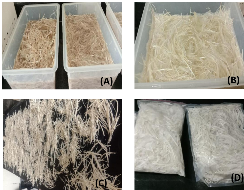
Fig 3.2 (A): Feathers soaked in detergent; (B): Feathers soaked in petroleum ether; (C): Drying of feathers in sunlight; (D): Stored clean feathers in plastic bags
