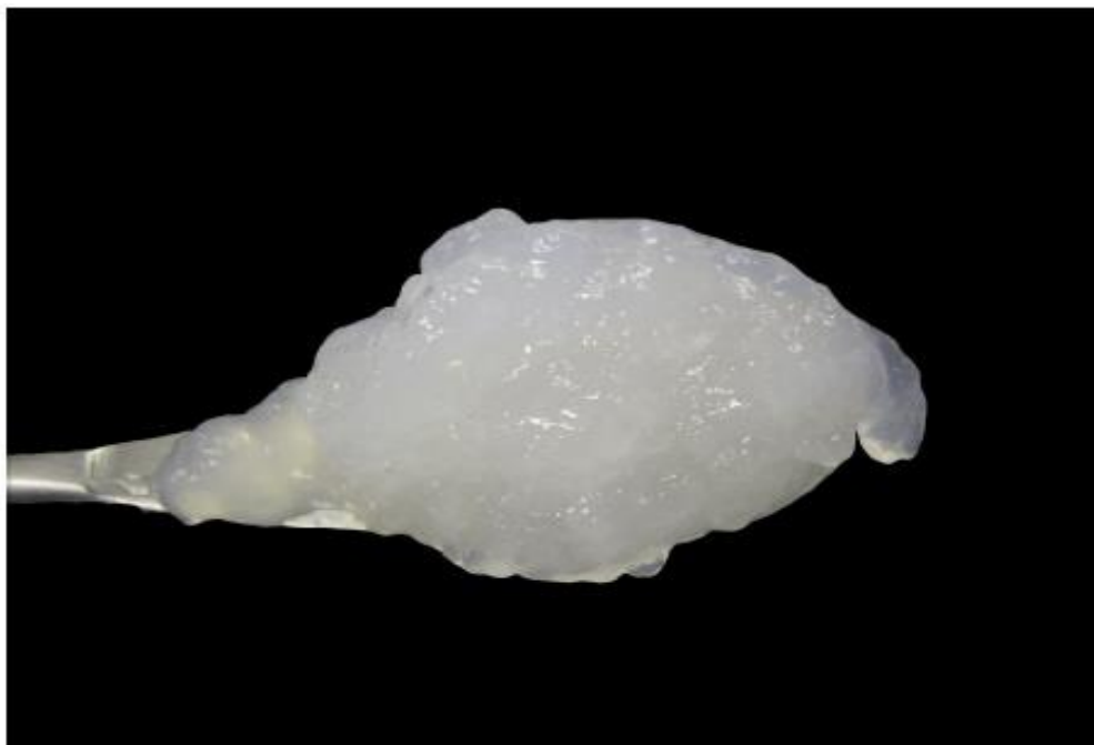
Fig. 6 Picture of a 2 w/v % micro fibrillated cellulose aqueous suspension from eucalyptus, enzymatic pre-treated [25]
