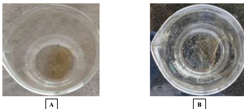
Figure 4.11: Biopolymeric film in control condition. A is 1 st day film in an open beaker. B is 30 th day film.
