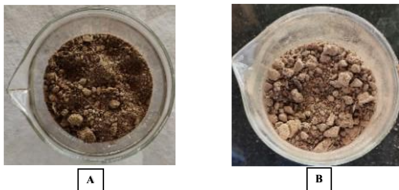
Figure 4.15: Biopolymeric film in dry soil sample. A is film before degradation at day 1. B is film after degradation at day 14.
