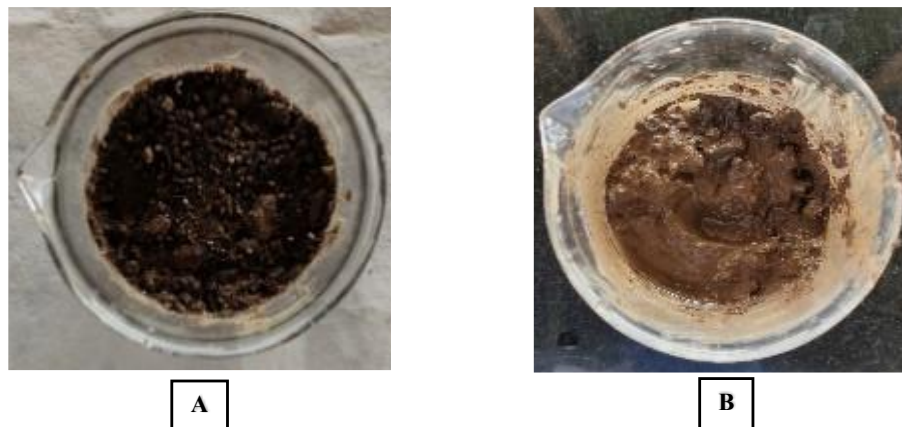
Figure 4.14: Biopolymeric film in daily wet soil sample. A is film before degradation at day 1. B is film after degradation at day 2.
