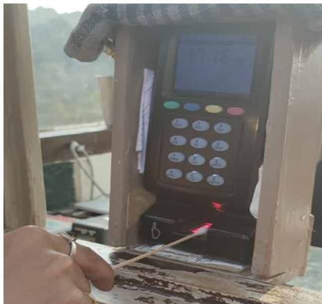
Fig 11 – Cotton swab rubbed on the scanner for sample collection.
