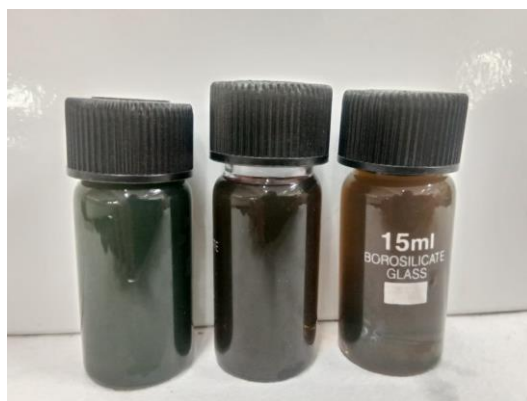
Fig 4.7 shows - The colour change in different pH after 24hr of catalytic reduction. pH 6, pH 7 and pH 8 respectively.
