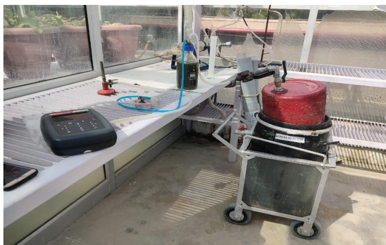
Figure 4.1: In this picture biogas is passed through algae substrate.
