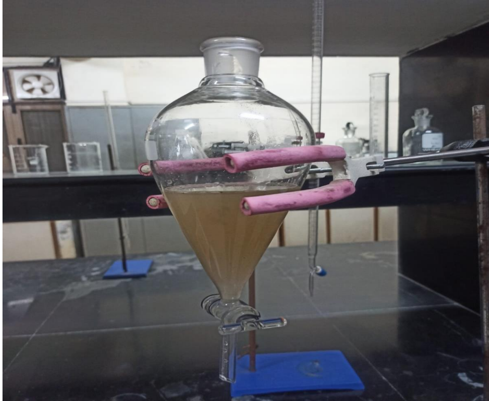
Figure 5.23 Oil and grease measurement using separating funnel.
