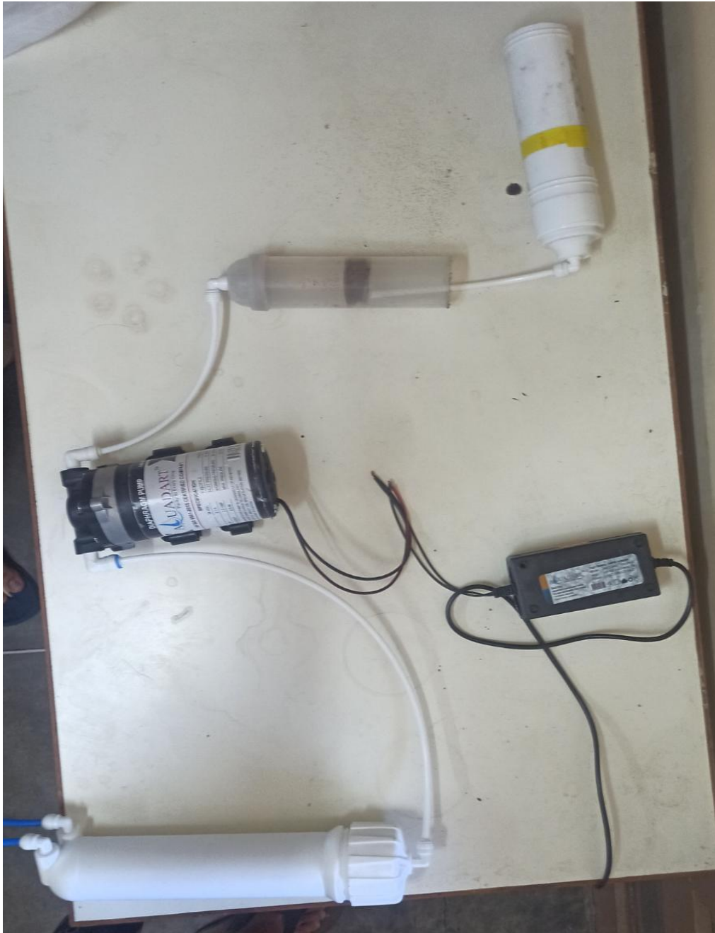
Figure 5.30 Prototype for automobile service centre waste water treatment.
