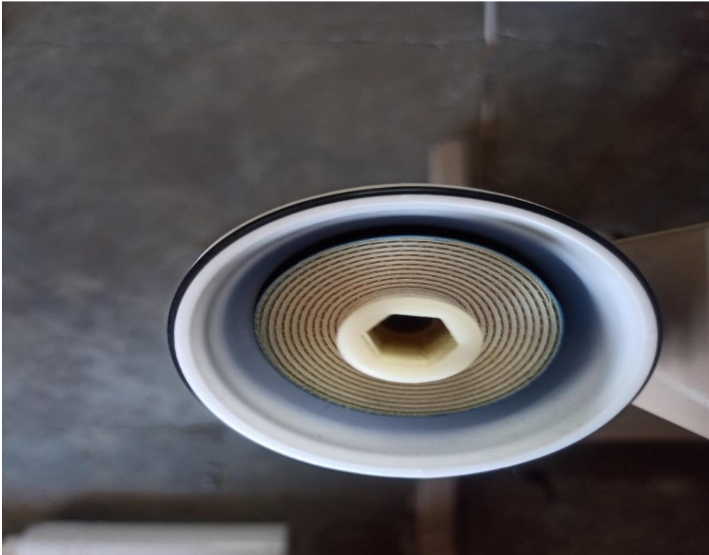
Fig 5.27 RO membrane used in prototype of waste water treatment.
